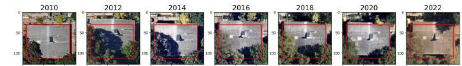
Fig. 1. A depiction of a roof with Super Six asbestos cement sheeting across seven time points, illustrating the geometric and illumination inconsistencies, as well as the impact of overgrown trees and shadows. The red polygon marks the building's location in 2010, emphasizing the misalignment of the building positions in subsequent years. (For interpretation of the references to colour in this figure legend, the reader is referred to the Web version of this article.)
