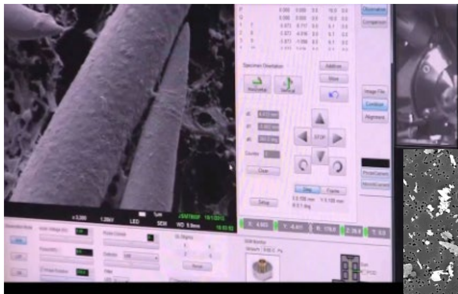
SEM image of a glass fiber collected on a polycarbonate filter.
