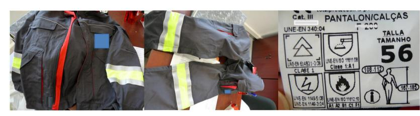
Example of thermal protective clothing with high-vis elements added after certification
