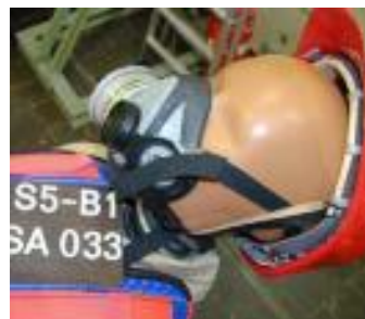
Figure 2: displacement of helmet, loss of filter, chin strap exerts pressure on throat
