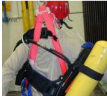
Figure 4: displacement of straps, position of breathing apparatus, straps cutting into neck area
