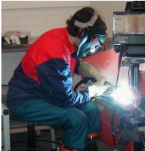
Figure 1. Eye and face protection against strong optical radiation is required by the Directive
