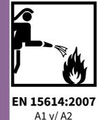
Codes included in the pictogram, A1, A2 or both, indicate the test method (Surface ignition or edge ignition, respectively), that has been carried out for determining the flame spread resistance.
