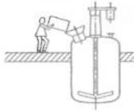
4. Big-bag discharge by gravity
